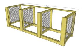
Screw a 2" x 4" x 10' stretched to the top of the back edge of the dividers using 2½" screws. The stretcher will provide structural support for the back of the compost bin.
