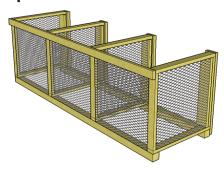
Remove the stretcher board and put it on top edge of the backside of the compost system, over the hardware cloth. Then using a hammer and 1" fence staple nails, attach the hardware cloth to the stretcher board.
