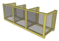
Attach hardware cloth to the back of the compost bin, starting on one end of the bin. Use a hammer to attach the hardware cloth with 1" fence staple nails.
