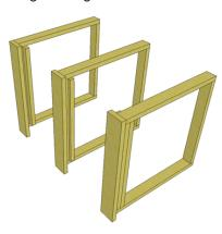
The  $2'' \times 6'' \times 39''$  are screwed to the front of the dividers using  $2 \frac{1}{2}''$  screws. Note: Three-four screws spaced evenly per board will be plenty. The front guides will have the same overhang as the inside guides. They will also be flush with the top of the square and overhang the bottom in the fashion shown in the images above.
