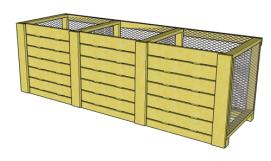
To complete your three-bin compost system, slide six door boards in the guide slots of each of the three bins. The spacers allow airflow in the front.
