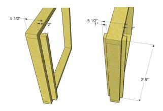
The 2" x 6" x 33" are attached to the inside of the dividers using 2 ½" screws on one of the 2' 9" sides. Note: Three-four screws spaced evenly per board will be plenty. The end dividers will have a 2" overhang on the inside as seen in the above left image. The middle dividers will have a 1" overhang on both sides as seen in the above right image.
